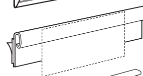
Clear Friction Fit Moulding with clear or foam tape
